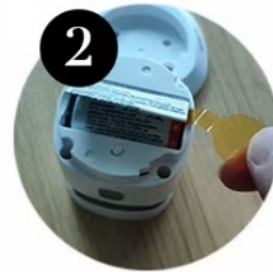
Remove the insulation
