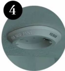
Screw the back plate Fixed to the wall
