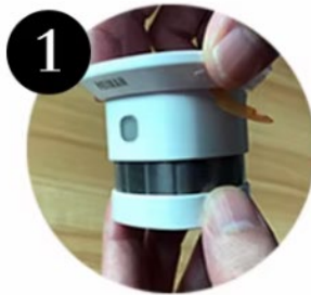
Remove the smoke back panel
